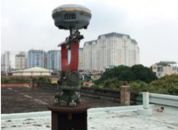
Figure 2.7. Accuracy testing equipment of GNSS - RTK technology
