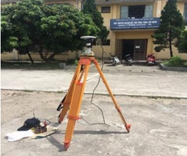
Figure 4.9. GNSS-RTK machine - mounted 360° mirror and 3G broadcasting system
